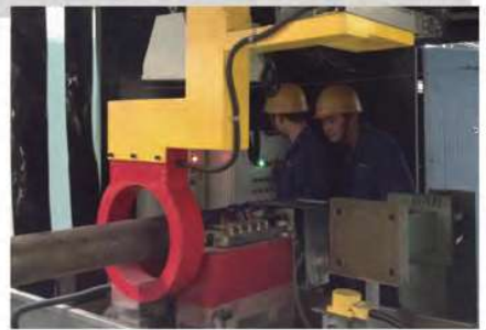
Pipe End Non-contact Multiple Vector MT System
