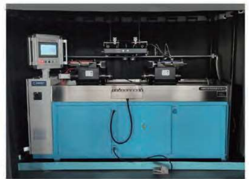
Standard Mag Bench with Automatic Spraying and Head Rotation
