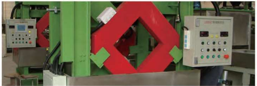
Square Bar in-line MT Station with Non-contact and Multiple Vector Functions
