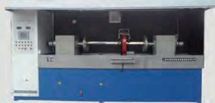
Standard Mag Bench with Steel Frame Hood
