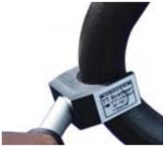
The ET system consists of the Ferroscope TT unit and a specialized scanner which, can inspect the vertical and horizontal sections of the tubes (including bends) in one run.
