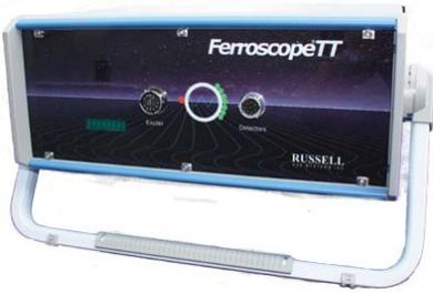
Russell group Systems has designed a sophisticated yet simple to operate ET system that effectively detects magnetite exfoliation flakes.
