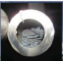
Russell Group has provided a solution, using through transmission (TT) electromagnetic technique for the detection and quantification of magnetite blockage in stainless steel tubes.
