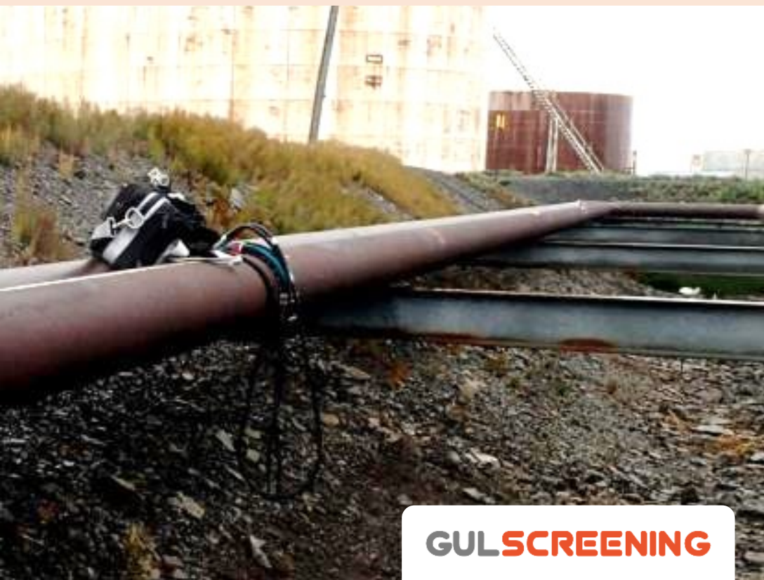
Photo of GUL Screening equipment on pipeline.
